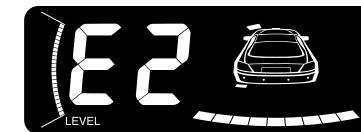
Example 2 Two sensors are damaged, they're sensor A and E.
